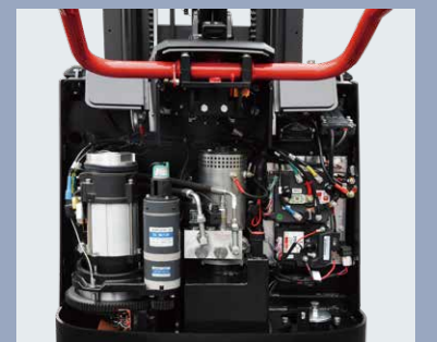
Back cover can be opened fully, and all components and parts are clear at a glance, which is very convenient for maintenance of the entire machine
