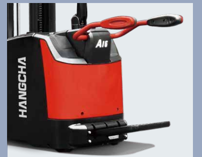
The integrated stamping molded guardrail offers better protection for the operator
