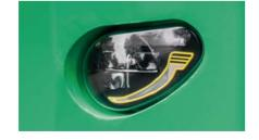
The whole vehicle is equipped with LED, and the integrated headlamps have daytime running lamps, far/near light, front turning streamer and other functions.
