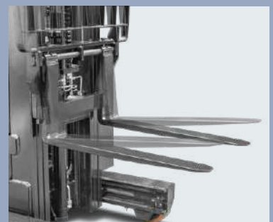
Forks can tilt forward/backward for easy loading
