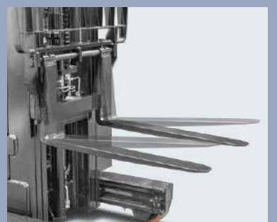
Forks can tilt forward/backward for easy loading
