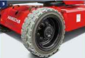
Tires: foam-filled tires with good off-road performance.
